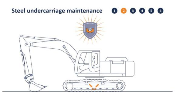
Roller guards extend the endurance of all components additionally. Mounted and maintained properly guards will improve the part's service life.
