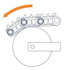
Pay attention to the track's running direction. Links have to pass the idler with the pin boss first.
