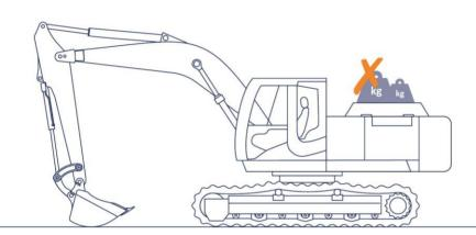
Added weight of attachments and counterweights increases wear.
